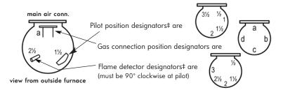
**Arrangement Designators** are specified relative to the main air connection at 12 o'clock and should be listed for **pilot**, **gas connection**, and flame detector in that order.
